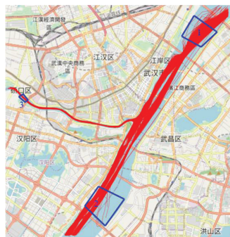
Figure 3. Schematic diagram of AIS trajectory after cleaning.
