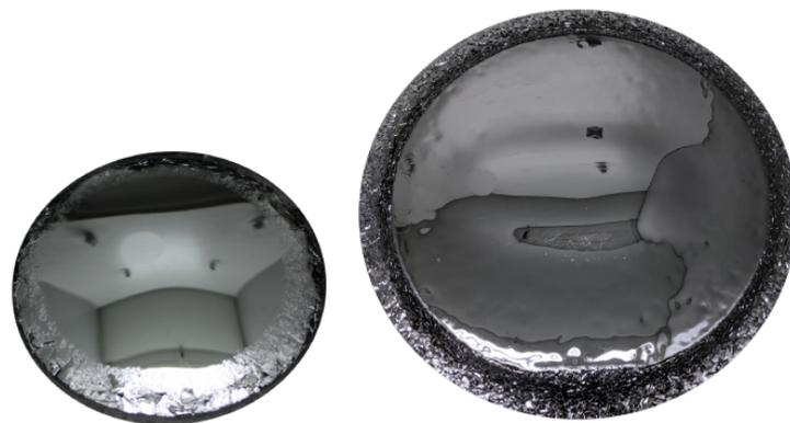
**Figure 14.** 100 mm (left) and 150 mm (right) 4H-SiC crystal.
