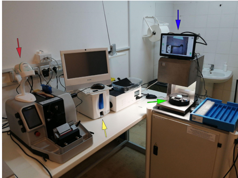
Figure 7. An example of a sectioning station. The technician can identify the block through a barcode reader (red arrow), entering the LIS page of the case and printing the related glass slides with a laser printer (yellow arrow). After sectioning, the technician can directly scan the cut surface positioning the block on the dedicated space in the BlocDoc instrument (green arrow), with the possibility to assess the preview of the obtained image (blue arrow).
