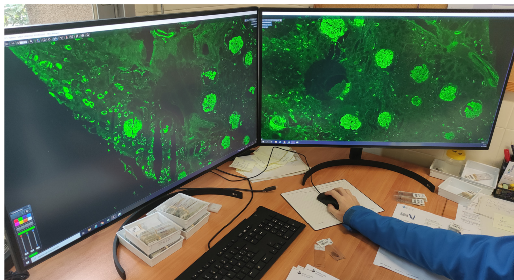
Figure 10. Fluorescence seen in a totally integrated fashion on two 32-inch LG 32HL512D 8MP diagnostic monitors.
