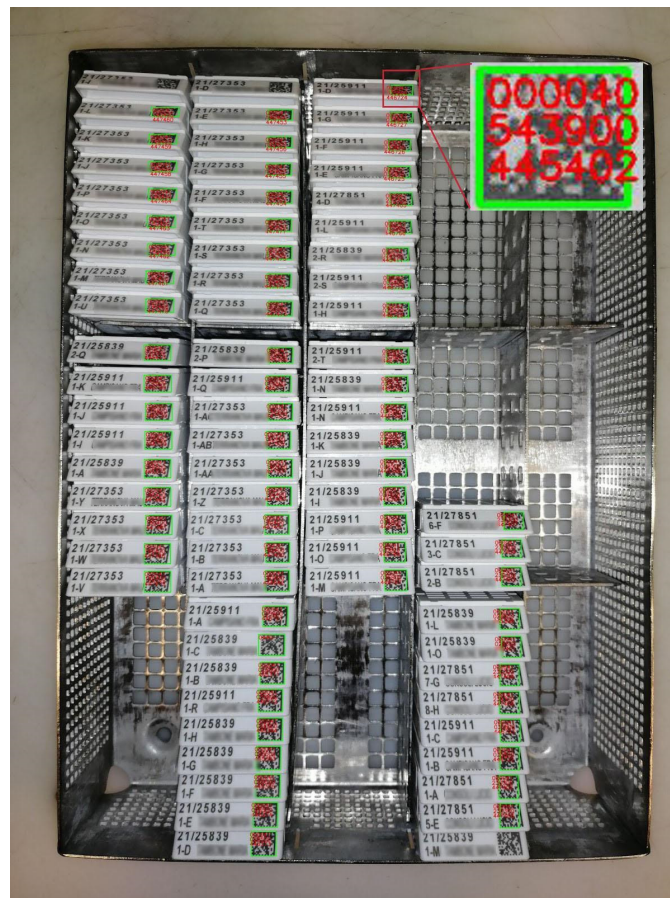
Figure 5. The reading process of barcodes directly from the rack containing the blocks during the processing phase after the digital transition. In the upper right inset the code extracted from the 2D barcode directly in the LIS.
