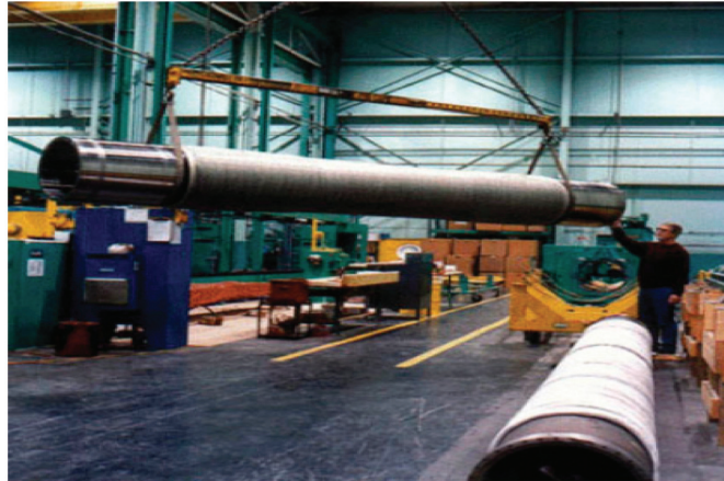
Figure 19. Composite riser pressure test samples (Courtesy of Lincoln Composites).
