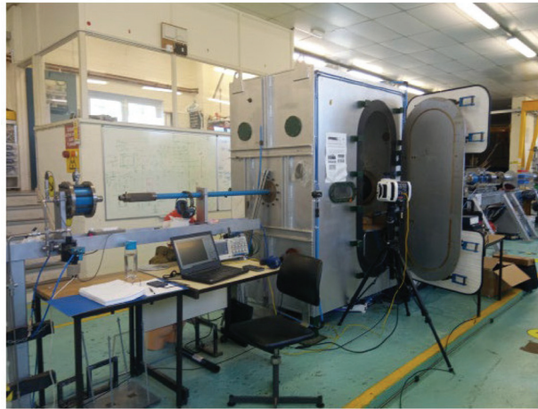
Figure 2. Picture of the setup for the gas gun and chamber.
