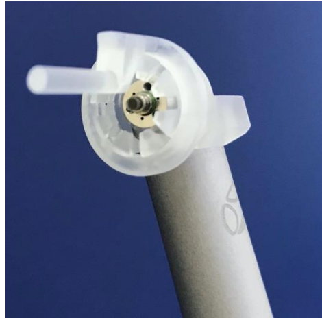
Figure 1. Adjustable rotating spacer, providing tip-to-tissue distance of 10 mm from 1.3 \times 6.3 mm sapphire tip, used in this study.
