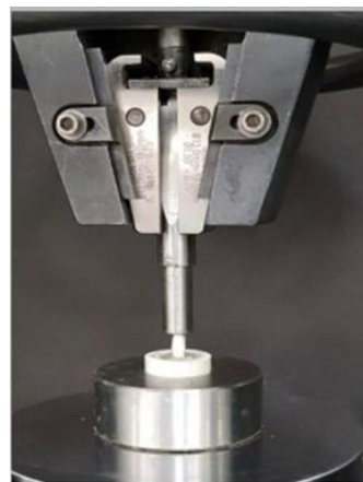
Figure 2. Fracture resistance test using Universal Testing Machine.
