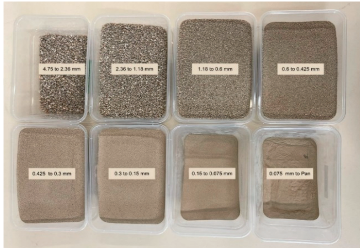
Figure 1. The coarse soil (B-sand) is sieved and separated into different containers depending on the granular size.
