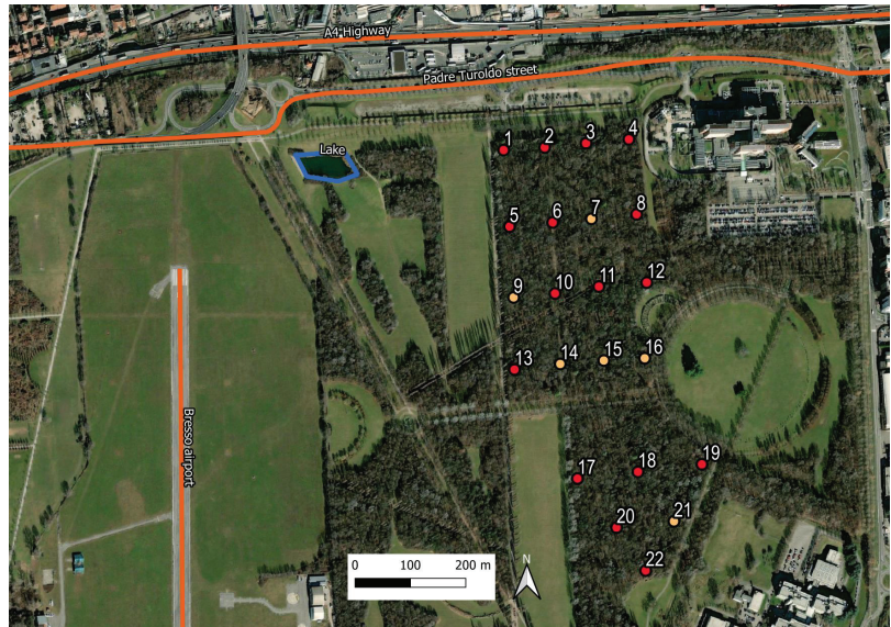
Figure 1. The Parco Nord (Northern Park) area of study. The sensor network is indicated by the numbered dots (1–22), deployed inside the tree-covered zone of the park. The network consists of two regular grids, the northern and the southern ones, composed of 16 and 6 nodes, respectively. Those in red color are the actually used sensors (total number 16), while those in yellow are the six ones discarded due to malfunctioning. One can see the A4 highway, the Padre Turoldo street and the artificial lake to the northern part of the park, while to the west side of it, the small Bresso airport runway is located.
