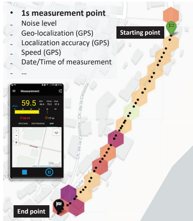
Figure 1. NoiseCapture approach. Using the NoiseCapture application, a user moves along a path (i.e., a track in the NoiseCapture vocabulary); each second (i.e., a measurement point), several noise indicators (sound level, spectrum) and other information (date/time, localization, speed, etc.) are calculated. When the user stops the measurements, the data are stored within the smartphone, and, if authorized by the user, uploaded to the NoiseCapture remote server. Raw data collected by the entire NoiseCapture community is preprocessed and averaged in hexagonal spatial zones (15 m radius); then, they are displayed in the form of noise maps.
