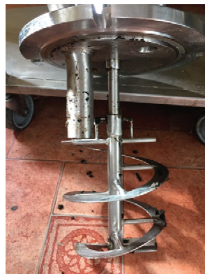
Figure 2. The geometry of the helical ribbon impeller used in this study.
