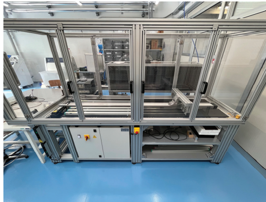
Figure 6. Stress-test machine employed to induce wearout in the resistive track and sliding cursor.
