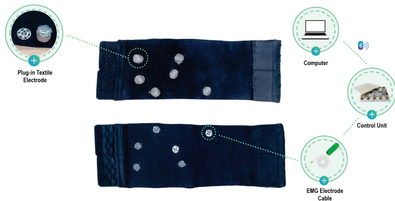
Figure 4. Smart textile sleeve: the upper part shows the internal view of the textile electrodes, while the lower part shows the external view connected to the acquisition system.
