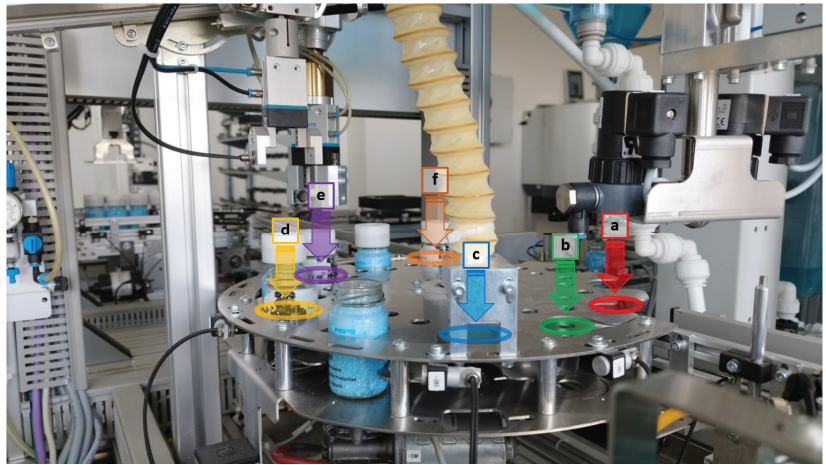
Figure 5. Filling Station of AFB Factory—(a) bottle entry; (b) liquid filling; (c) granulate filling; (d) cap placing; (e) cap closing; (f) bottle exit.
