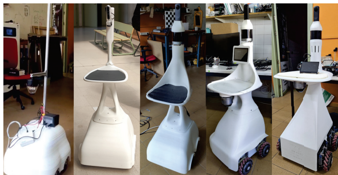
Figure 2. Evolution of the Shadow robot. From left to right: The different phases of the construction of the Shadow robot, from its initial version to its final version, with an omnidirectional base and a touchscreen for interaction.
