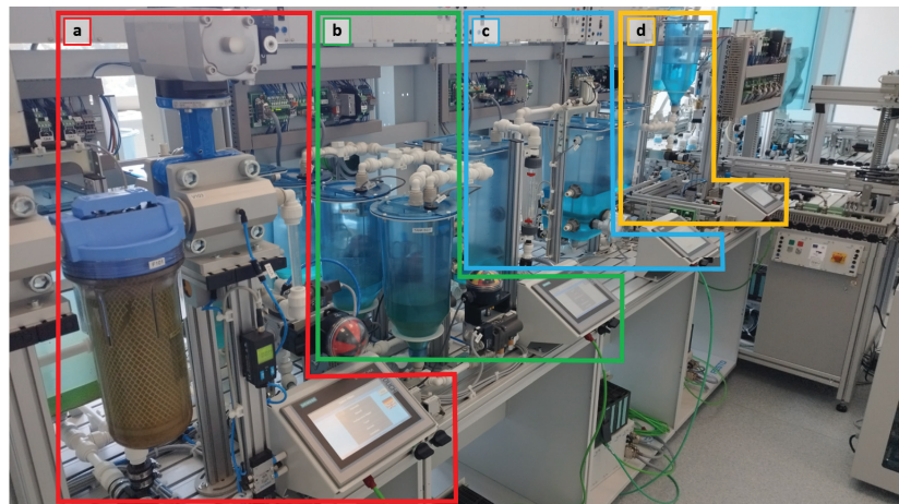
Figure 8. Liquid material preprocessing in AFB Factory—(a) liquid filtering; (b) liquid mixing; (c) liquid heating; (d) liquid quality check.
