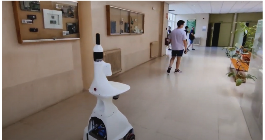
Figure 13. A screenshot of Shadow following a person, maintaining a safe distance, and demonstrating smooth movements of its omnidirectional base ( https://youtu.be/_vndgz-sviE , accessed on 22 August 2024).
