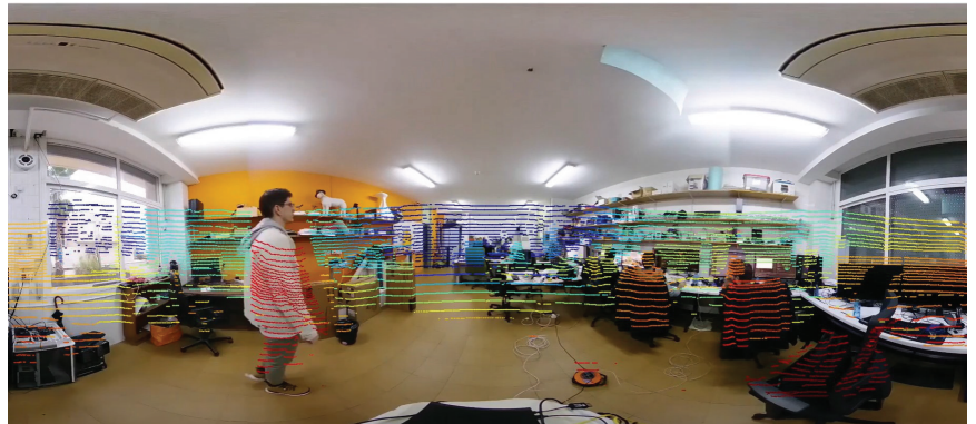
Figure 12. Output from the 360° RGB camera with LiDAR depth overlay on a jet colormap, demonstrating the calibration results. The colors represent different depth levels, with warmer colors indicating closer distances and cooler colors indicating farther distances.
