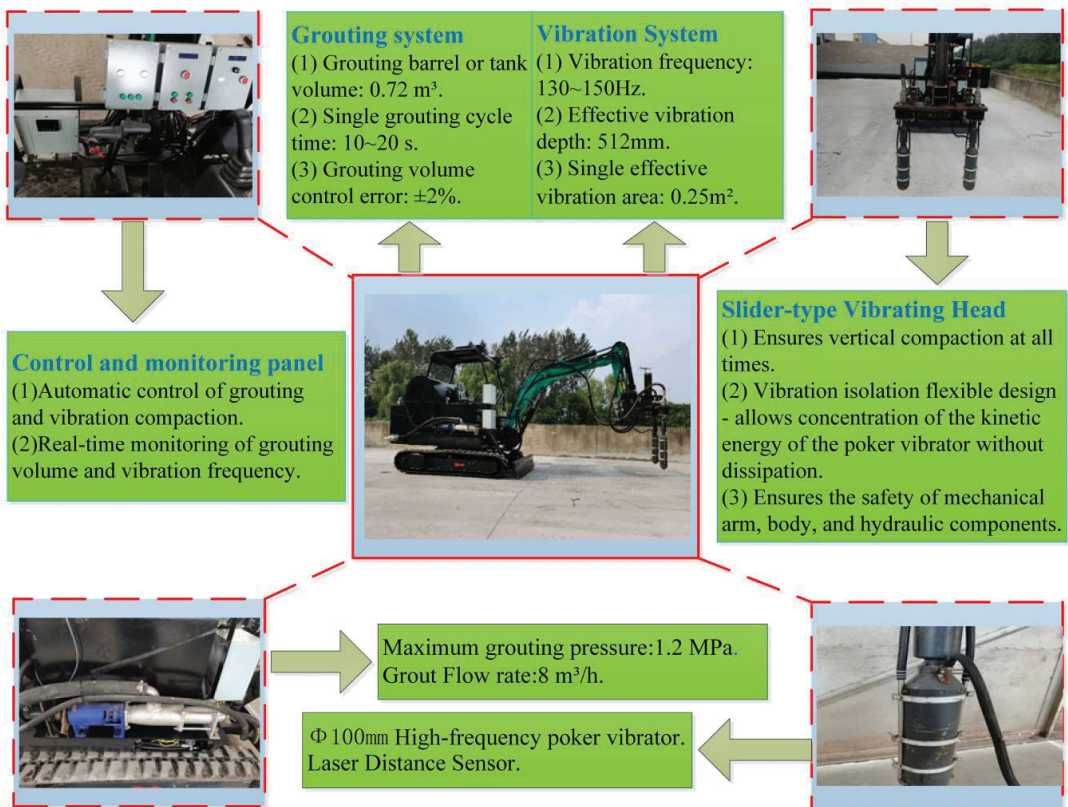
Figure 8. The grouting and vibrating equipment of CSGR.
