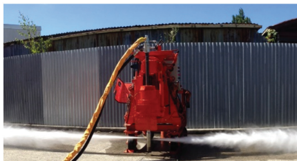
Figure 8. Jet grouting machine (courtesy of the Chemical Grouting Co., Ltd., Tokyo, Japan).
