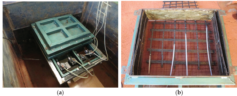
Figure 3. Small-scale pullout test apparatus: (a) overall view; (b) inextensible wires over the GGR length.
