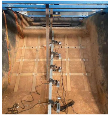
Figure 5. Wooden frame beam–bamboo anchor slope model test front.
