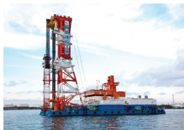
Figure 11. A new deep mixing vessel (courtesy of the Toa Corporation, Tokyo, Japan).
