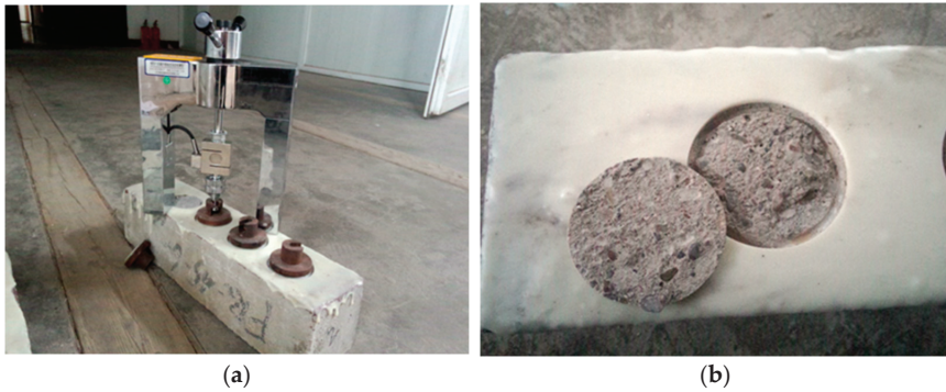
Figure 6. Pull-out test of structural adhesive: (a) Pull-out test; (b) Typical case after failure.
