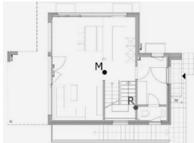
Figure 2. An example of dislocation between the centre of gravity (M) and the centre of rigidity (R), [16].
