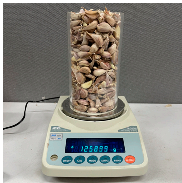
Figure 7. Bulk density measurement.
