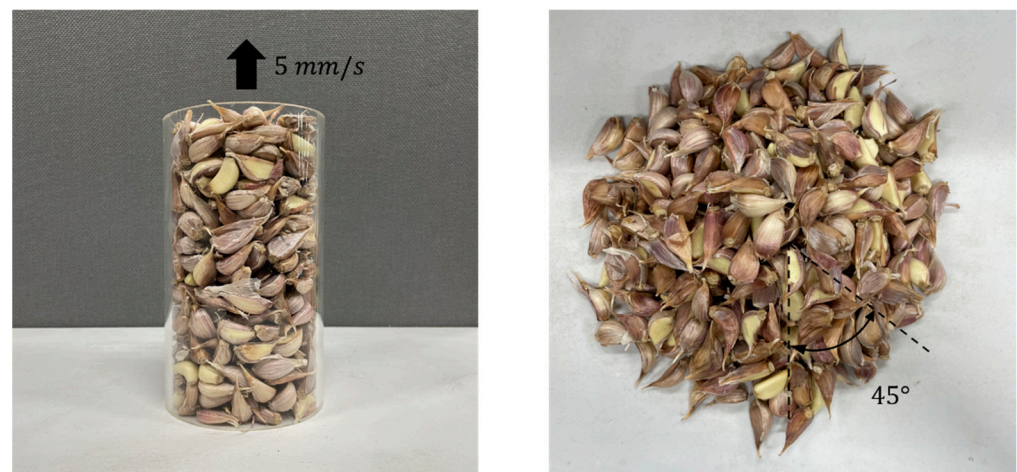
Figure 9. Repose angle test.
