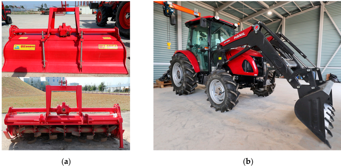
Figure 2. Tractor–implement system used in this study: (a) rotavator (WJ185A, Woongjin, Republic of Korea); (b) 42 kW class agricultural tractor (TX58, TYM, Gongju, Republic of Korea).
