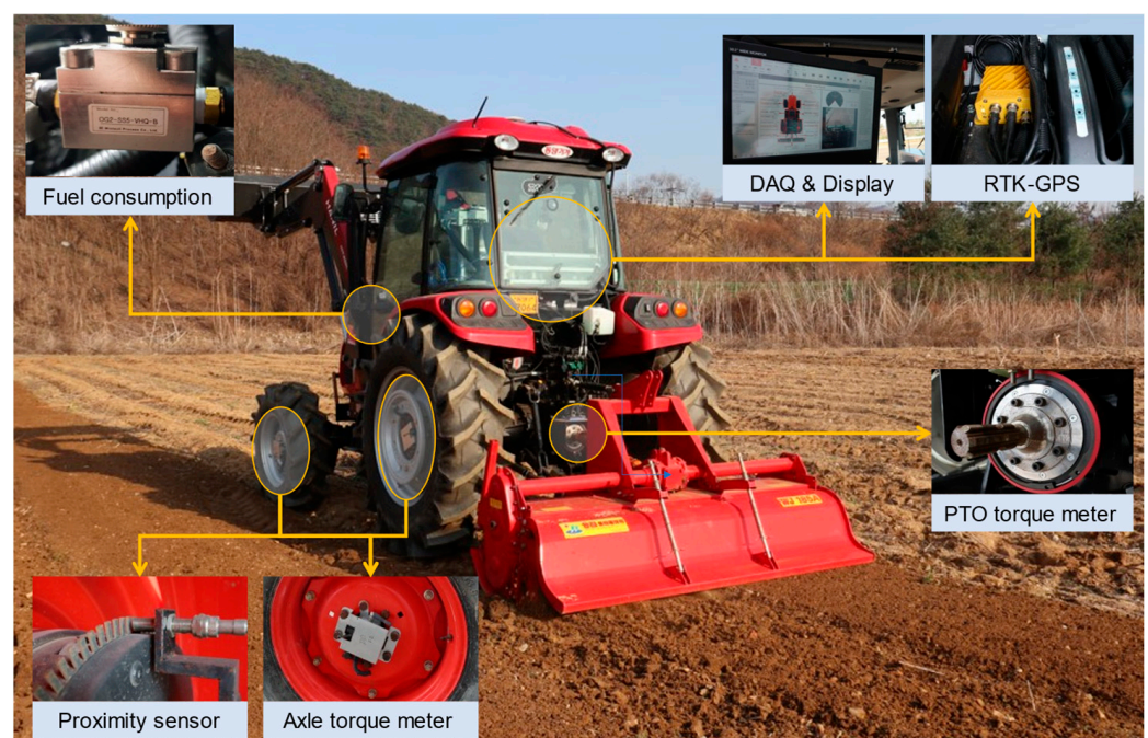
Figure 3. Configuration of the field load measurement system.
