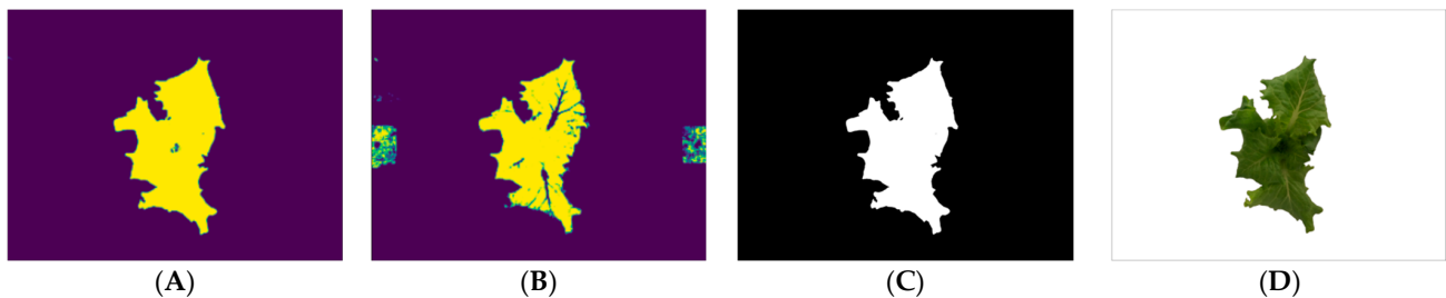
Figure 7. Additional image processing to acquire images of the ROI: (A,B) noise removal through Lab color system, (C) binary image, and (D) mask image.
