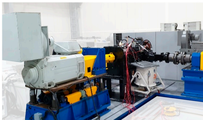
(b) photograph of the 3-axis dynamometer system
