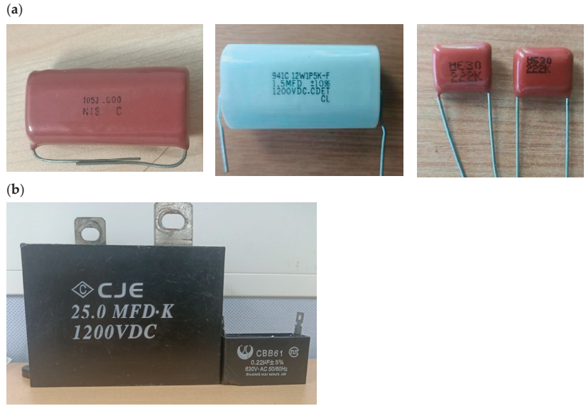
Figure 3. The digital images of film capacitors. (a) Wound-type film capacitors. (b) Stacked-type film capacitors. The capacitor on the left is used for DC circuits, while the one on the right is used for AC circuits.
