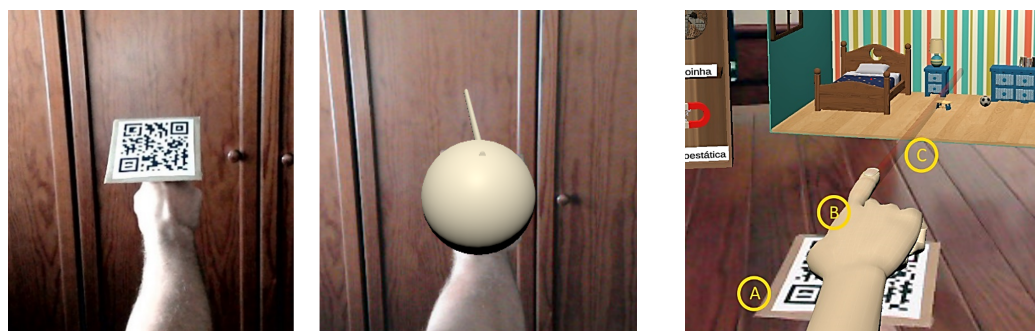
(a) Virtual wand. Left: input image; Right: input image augmented with virtual wand. (b) Virtual hand and laser. A: marker; B: hand; C: laser.
