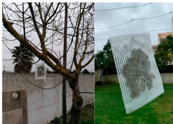
Figure 2. Exposed transplanted Flavoparmelia caperata lichens in nylon bags (right) that were placed in the study area (left).
