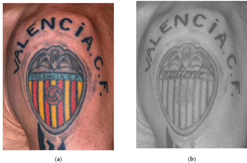
Figure 9. Images of tattooed shoulder: (a) captured with a conventional camera and illuminated with white visible light, and (b) captured by Invespector and illuminated with IR radiation 850 nm.
