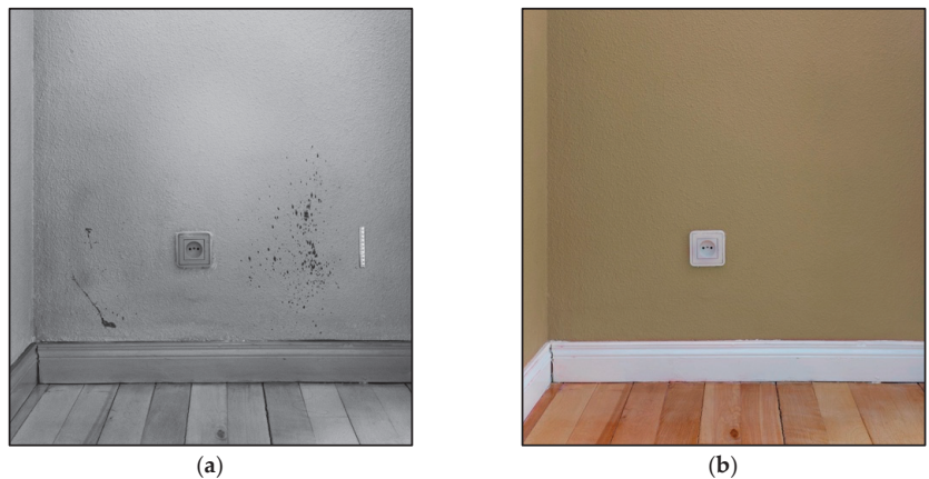
Figure 6. Images of a wall with traces of latent blood under a layer of acrylic paint: (a) photographed with a conventional camera and illuminated with white visible light and (b) by Invespector illuminated with IR radiation 850 nm.
