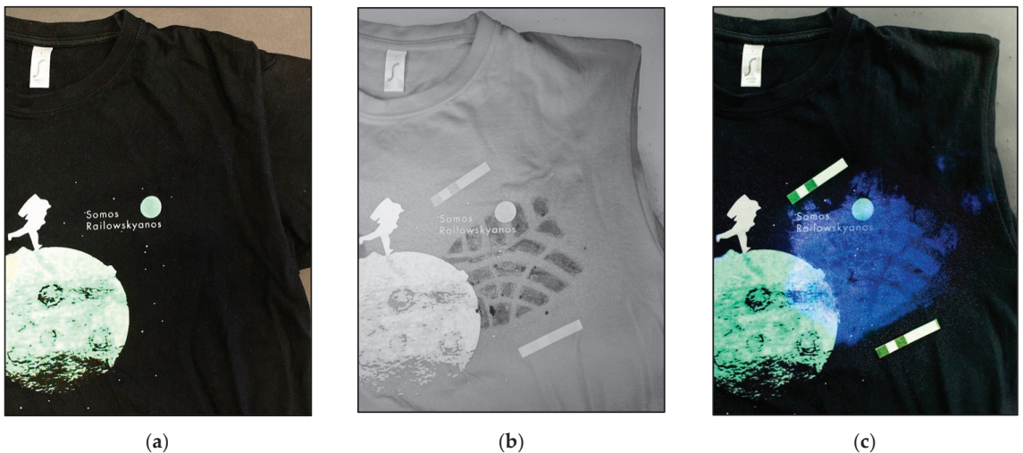
Figure 4. Images of black cotton shirt with traces of latent blood photographed (a) with conventional camera and illuminated with white visible light, (b) by Investigator illuminated with IR radiation 850 nm and (c) after applying a chemo locator, such as Bluestar.
