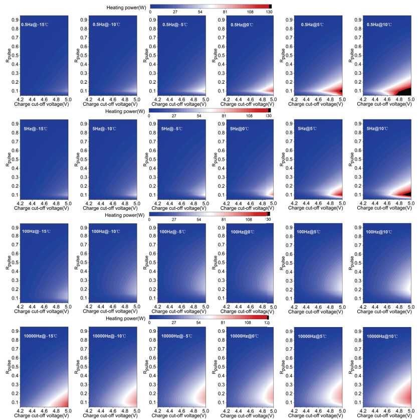
Figure 10. Variation of the relationship between R_{pulse} and heating power with frequency and temperature at different charge cut-off voltages.
