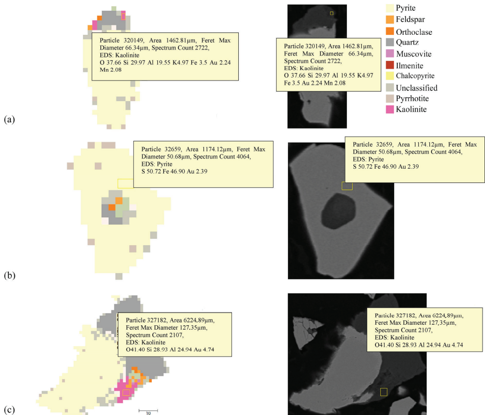
Figure 5. Occurrence of invisible gold inside mineral grains; (a) gold in kaolinite hosted using pyrite grain, 10 \mu\text{m} scale; (b) gold-inclusion pyrite, 5 \mu\text{m} scale; (c) invisible gold hosted using kaolinite, 10 \mu\text{m} scale.
