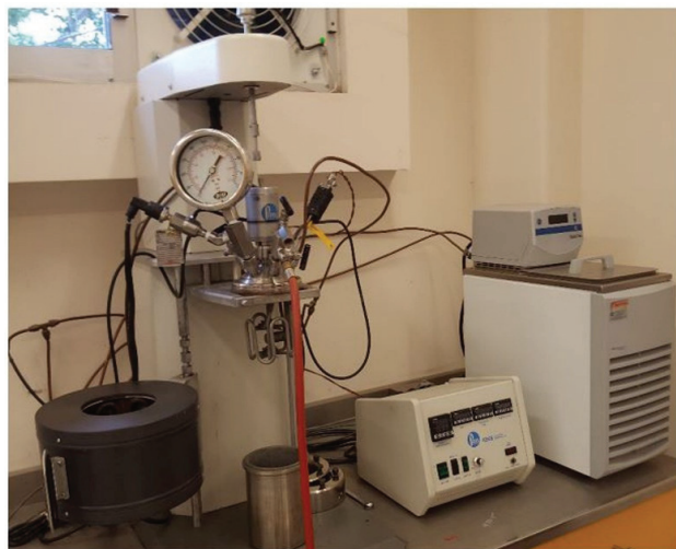
Figure 1. Experimental setup for simultaneous pressure leaching and oxidation.
