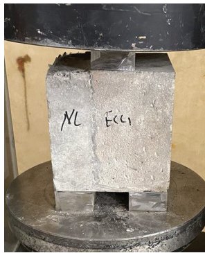
Figure 9. Bi-surface shear test and test setup.
