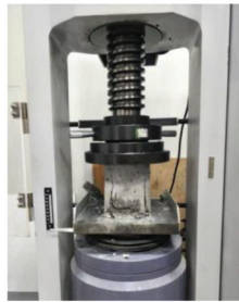
Figure 1. Compressive test for concrete.
