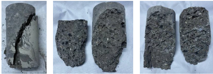
Figure 14. Slant shear typical failure mode C—Interfacial failure with a thick layer of the substrate.
