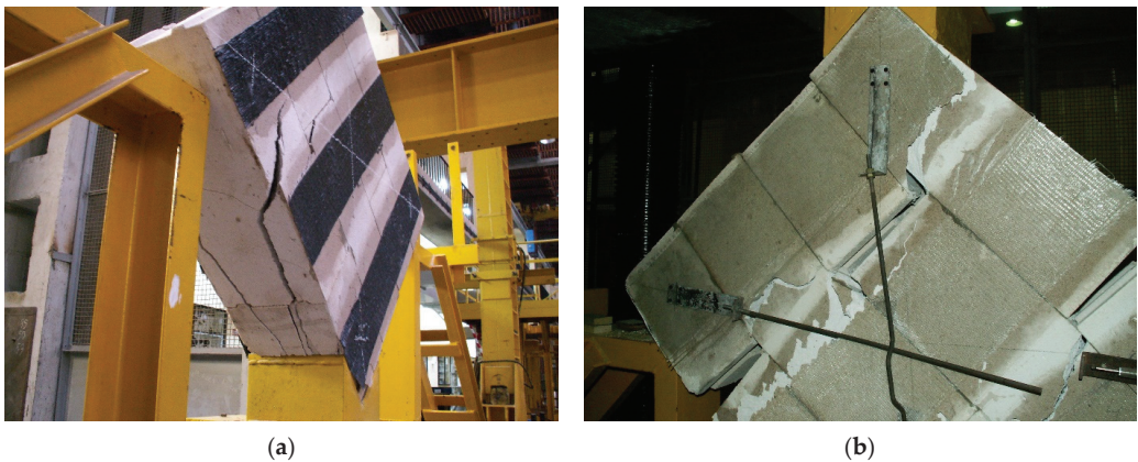
Figure 10. Failure pattern observed in walls strengthened in configuration ‘b’: (a) the elements with carbon strips; (b) the elements with glass strips.
