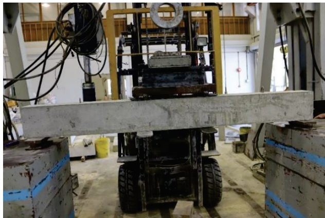
Figure 5. Experimental setup of RC beam specimen.
