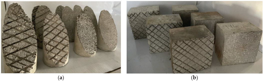
Figure 7. Interface roughness (a) half cylinder grooved and as cast surface and (b) two-thirds of the cube grooved and as cast surface.
