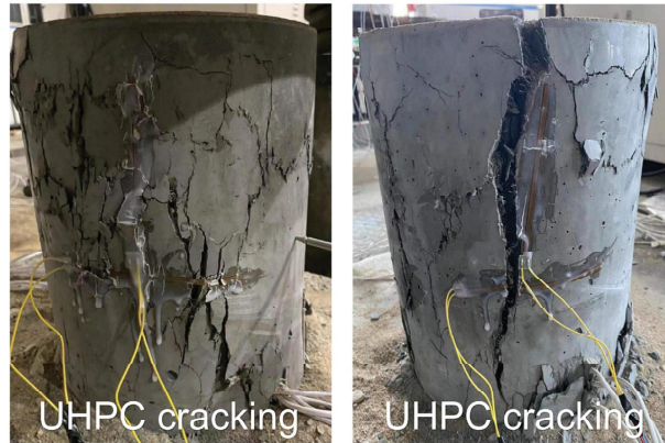
Figure 4. Z4 and Z5 failure forms.
