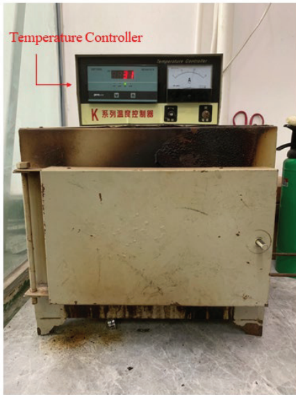
(a) Electric furnace
