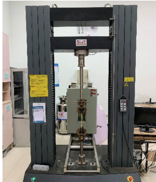
(b) ETM series electronic universal testing machine
