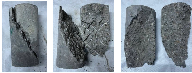
Figure 12. Slant shear typical failure mode B—Interface failure with a thin layer on the substrate.
