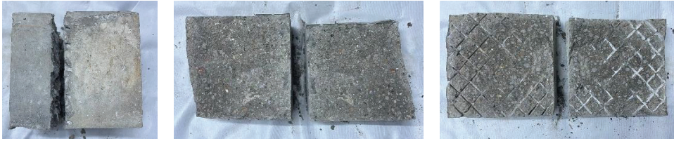
Figure 13. Bi-surface typical failure mode B—Interface failure with a thin layer on the substrate.
