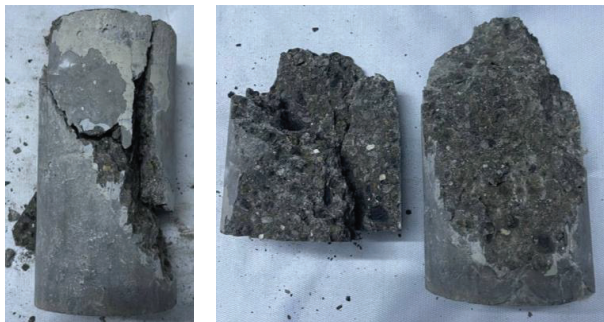
Figure 16. Slant shear typical failure mode D—Complete substrate failure.
