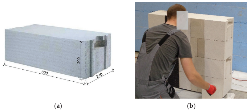
Figure 1. The view of element: (a) AAC block; (b) masonry wall before the application of strengthening.
