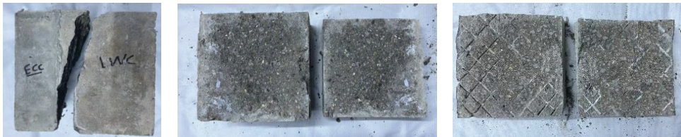
Figure 15. Bi-surface typical failure mode C—Interfacial failure with a thick layer of substrate.
