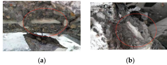
Figure 7. Observed damage of GFRP. (a) Outer rubber layer failure (BC-9); (b) Fiber bundle breakage (BC-3).
