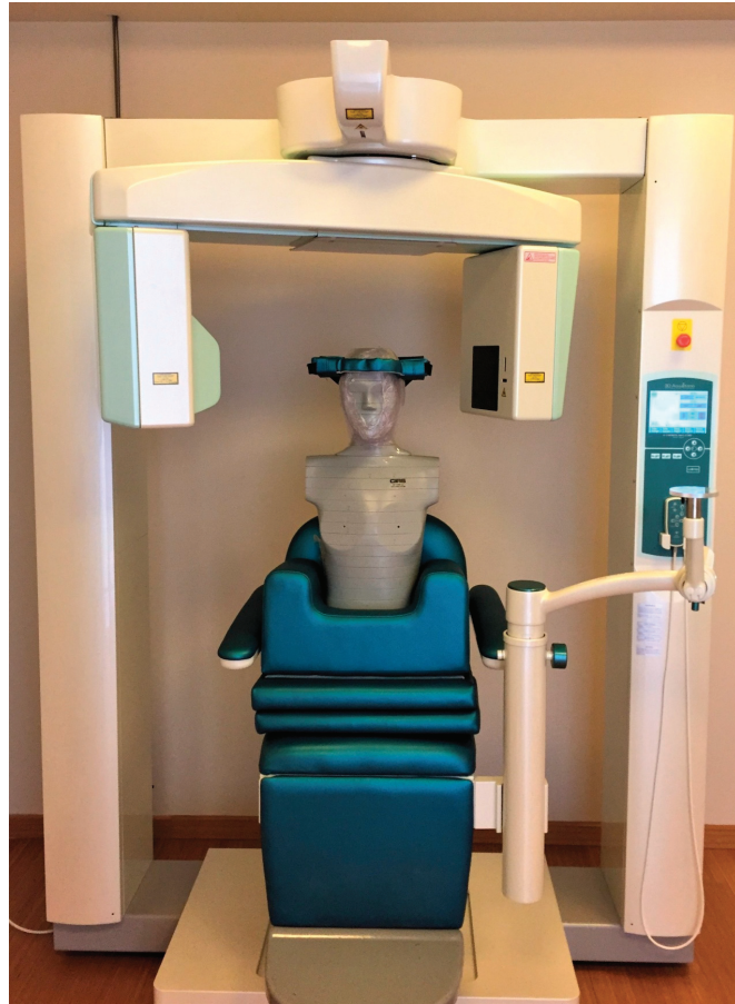
Figure 1. Anthropomorphic phantom (NATHANIA) was placed in the X-ray gantry of the cone-beam computed tomography (CBCT) device to imitate clinical conditions.
