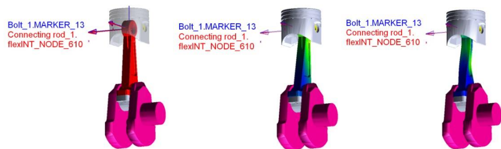
Figure 35. Snapshots during virtual simulations of the considered mechanism with a deformable connecting rod (MARKER_13 Node 610 location).
