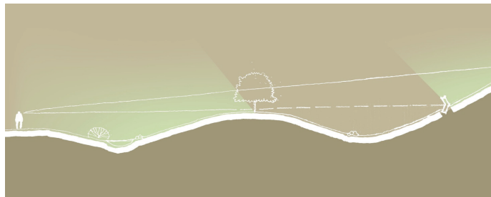
Figure 1. The area visible from the viewpoint may be blocked by vegetation, topography or other objects. A viewpoint is defined by its view direction, view width, and view distance.
