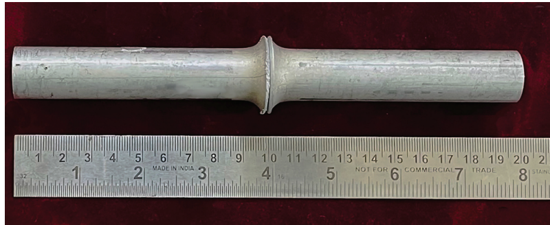
Figure 3. Visual view of rotary friction-welded AA5083 H116 joint.
