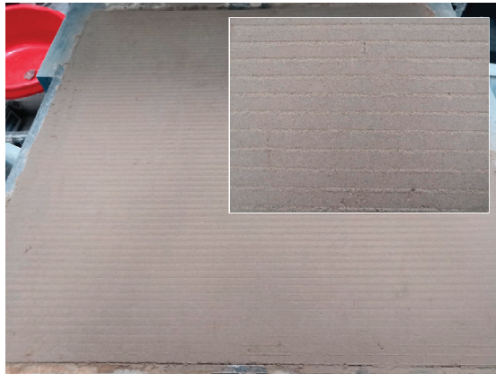
Figure 7. Shear interface after the test was completed.
