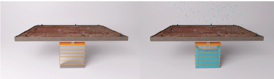
Figure 7. Visualization of the extensive green roof before and after the simulation. The total accumulated amount of runoff water to the stormwater tank is 7.25 m 3 .
