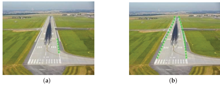
Figure 9. Correlation loss eliminates missed detection. (a) Missed detection line (without correlation loss). (b) High detection accuracy (without correlation loss).
