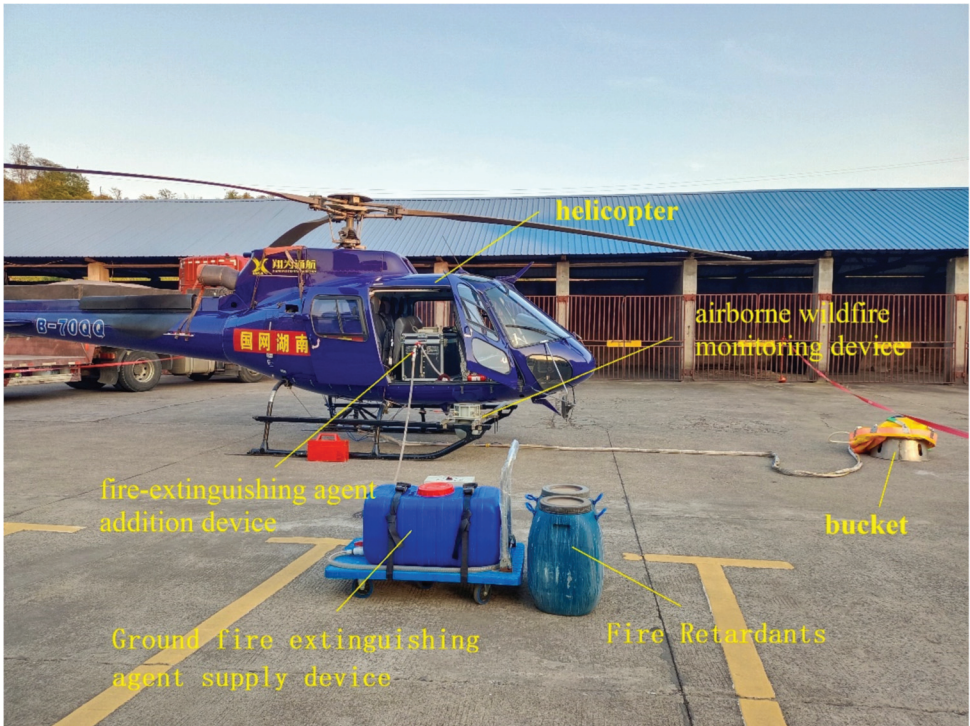
Figure 27. Adding a flame retardant to a firefighting helicopter.
