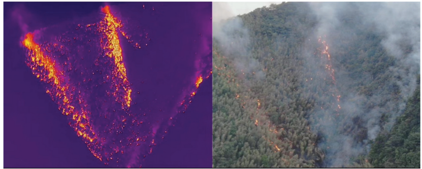
Figure 26. Monitoring map for the local location of on-site wildfires. Left image shows an infrared image of wildfire disasters and the right hand picture shows the visible light image of a wildfire disaster.
