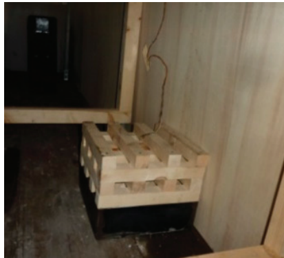
Figure 4. Wood crib/container assembly, including the container for water and accelerant (heptane).
