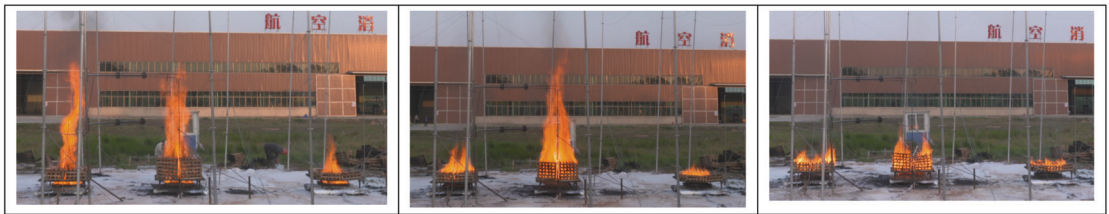
Figure 14. Combustion conditions of the fire scenes in the model using Agent#2 taken from the helicopter after spraying the flame retardant onto the wood crib. First subgraph: 180 s; second subgraph: 600 s; third subgraph: 870 s.
