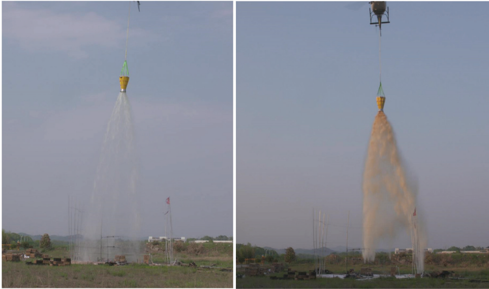
Figure 8. Helicopter high-altitude spraying of flame retardants. (Left): gel fire-extinguishing agent; (Right): class AB fire-extinguishing agent.
