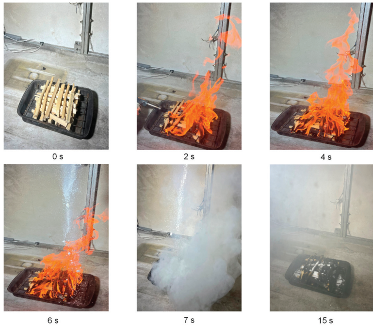
Figure 16. Snapshots of the suppression of a model wood crib fire with several tiers using carbon dioxide hydrate powder: m_g \approx 80 g.
