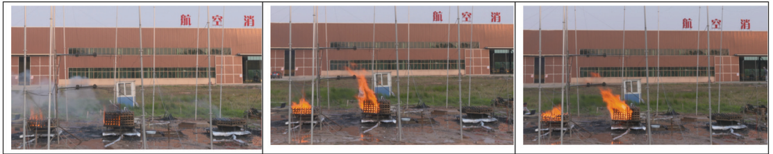
Figure 16. Combustion conditions of the fire scenes in the model using Agent#3 taken from the helicopter after spraying the flame retardant onto the wood crib. First subgraph: 180 s; second subgraph: 600 s; third subgraph: 870 s.
