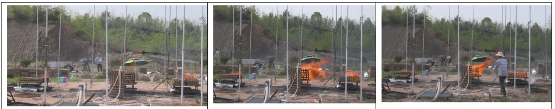
Figure 18. Combustion conditions of the fire scenes in the model using Agent#4 taken from the helicopter after spraying the flame retardants onto the wood crib. First subgraph: 180 s; second subgraph: 600 s; third subgraph: 870 s.
