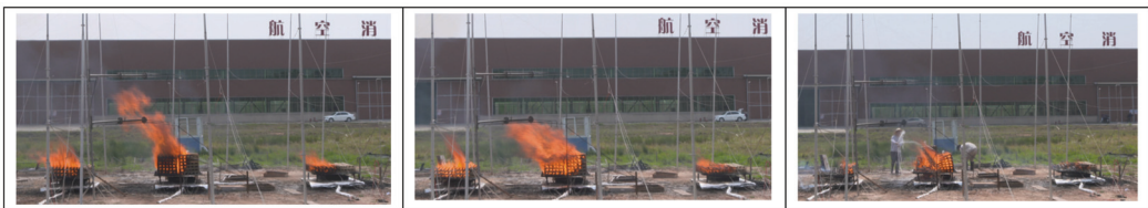
Figure 9. Combustion conditions of the fire scenes in the model without spraying flame retardants onto the wood crib. First subgraph: 180 s; second subgraph: 600 s; third subgraph: 870 s.
