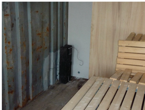
Figure 7. Hot-plate thermometer located in the corner (configuration C1).
