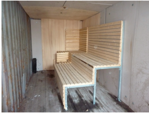
Figure 2. Test chamber: benches and drywall/plywood boards.
