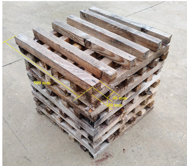
Figure 2. Photograph showing the construction of the 12-layer wood cribs.
