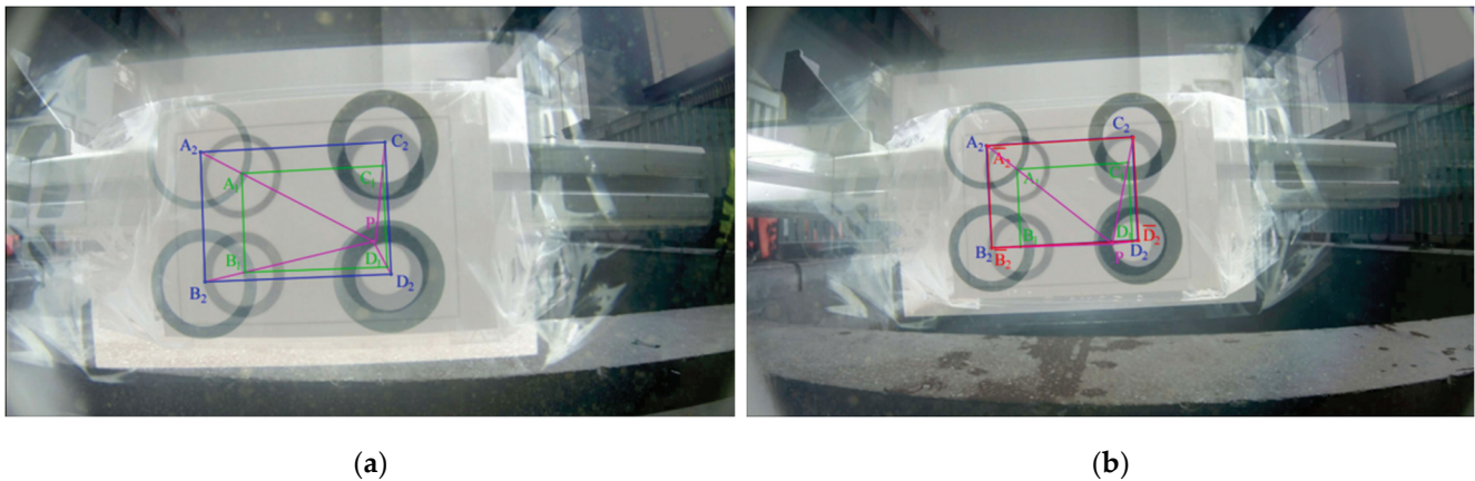
Figure 15. Projection of the same target on the imaging plane underwater and above water. (a) When D = 200 mm, record the same target's projection on the imaging plane underwater and above water and mark its keypoints. In this figure, A_1, B_1, C_1, D_1 represents keypoints of the above-water image, A_2, B_2, C_2, D_2 represents keypoints of the underwater image. (b) When D = 260 mm, the location of the underwater keypoints is predicted from the calculated value of K and compared with the actual value. In this figure, \overline{A_2}, \overline{B_2}, \overline{C_2}, \overline{D_2} represents predicted keypoints of the underwater image.
