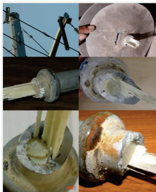
Figure 1. Illustrations of the damage, degradation and aging of polymeric insulators [11].
