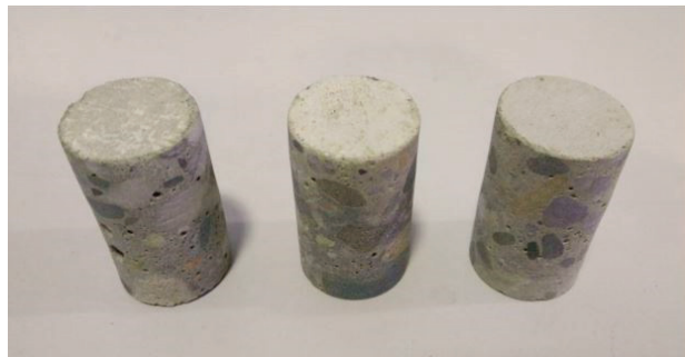
Figure 1. Concrete cores prepared for testing using X-ray computed microtomography.
