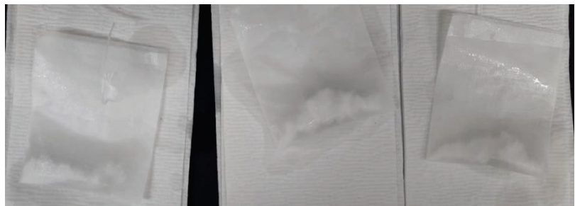
Figure 6. Gel blocking observed in the tea-bag method by SAP A in the first few minutes.
