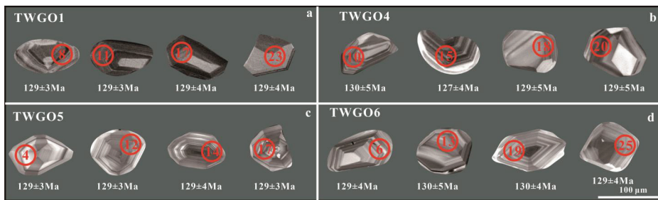
Figure 3. U–Pb zircons cathodoluminescence images from the volcanic rocks of the Longjiang formation at Lengjimanda plate. Circles indicate the locations of U–Pb analysis on zircons, along with their respective zircon numbers, and age information listed below. (a) TWG01, (b) TWG04, (c) TWG05, (d) TWG06.
