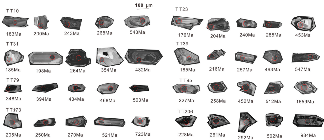
Figure 5. CL images of the analyzed zircons from the 8 meta-sedimentary rocks. Please see the main text for descriptions. Red circles denote the laser spots during the geochronological analyses.
