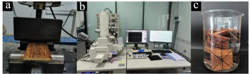
Figure 2. (a) MOR and MOE testing, (b) scanning electron microscope and (c) dimensional stability test.
