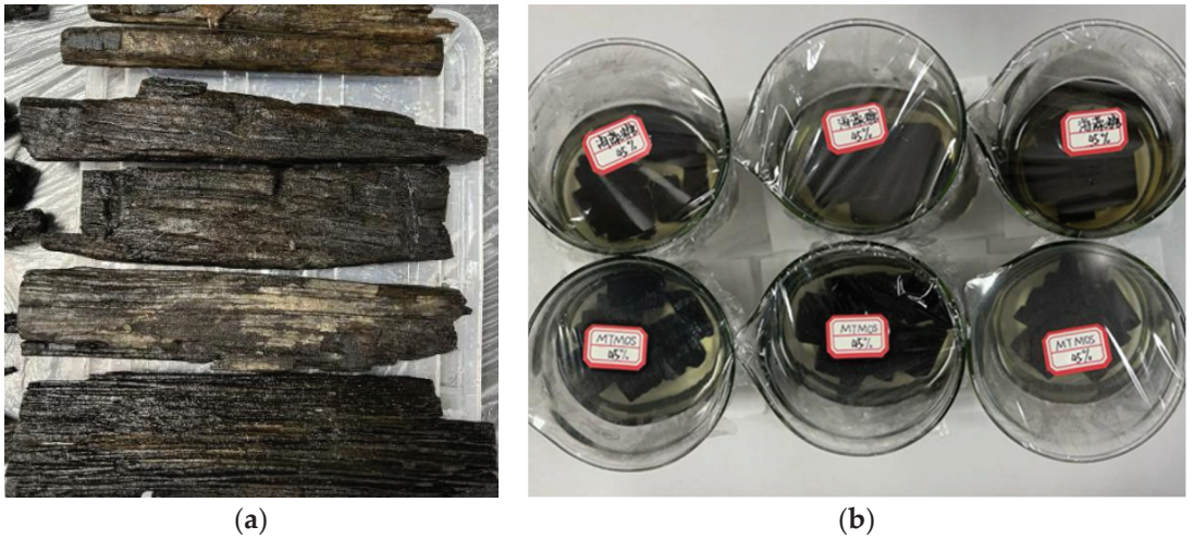
Figure 1. Samples from the ancient ship “Luoyang Canal No. 1” (a) the excavated ship planks and (b) samples submerged in consolidants. Note: The Chinese word “海藻糖” in the (b) means trehalose.
