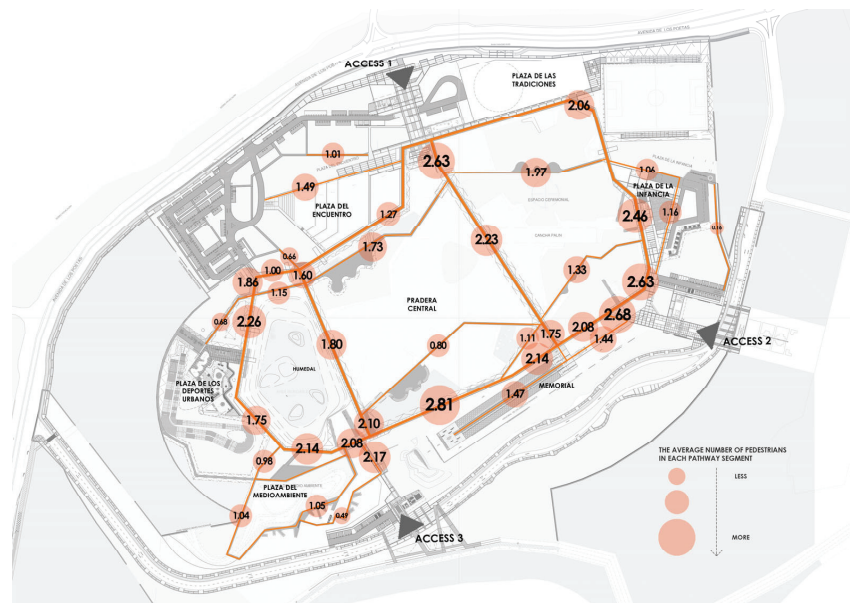
Figure 5. Average number of pedestrians on road segments (number of road segments: 39).
