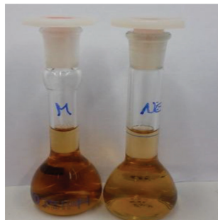
Figure 5. Extracted solutions obtained using the two extraction methods: M: Maceration; NE: RSLDE 1030 cycles.
