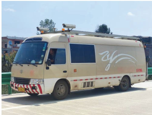
Figure 4. RTM-type vehicle-mounted intelligent road detection system.
