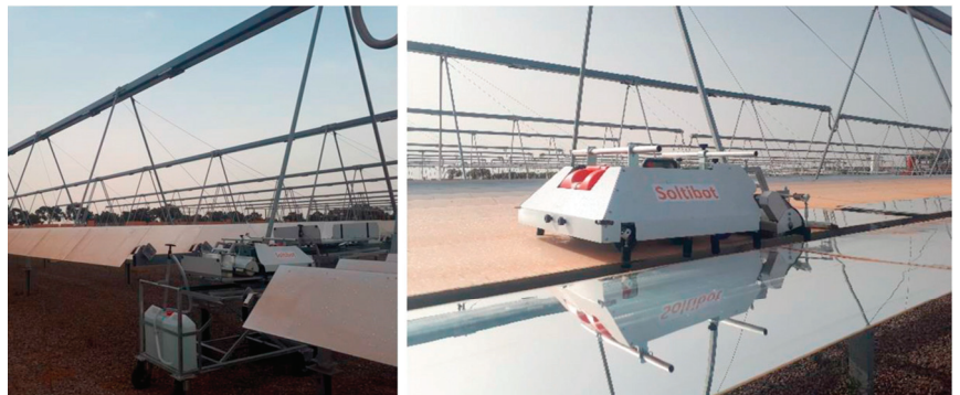
Figure 1. Cleaning event; left: the selected collector on dirty state, right: operating cleaning robot on the day of cleaning [36].
