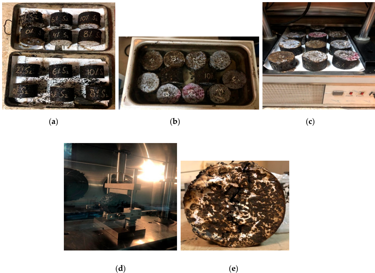
Figure 11. Moisture susceptibility testing: (a) Unconditioned samples 's-1' and conditioned samples 's-2'; (b) Conditioning of samples in water bath for 24 h at 60 °C; (c) Unconditioned and conditioned samples kept at 25 °C for 4 h in a temperature-controlled chamber prior to testing; (d) Samples tested in UTM where the load was applied at 50 mm/min; (e) Fractured sample.
