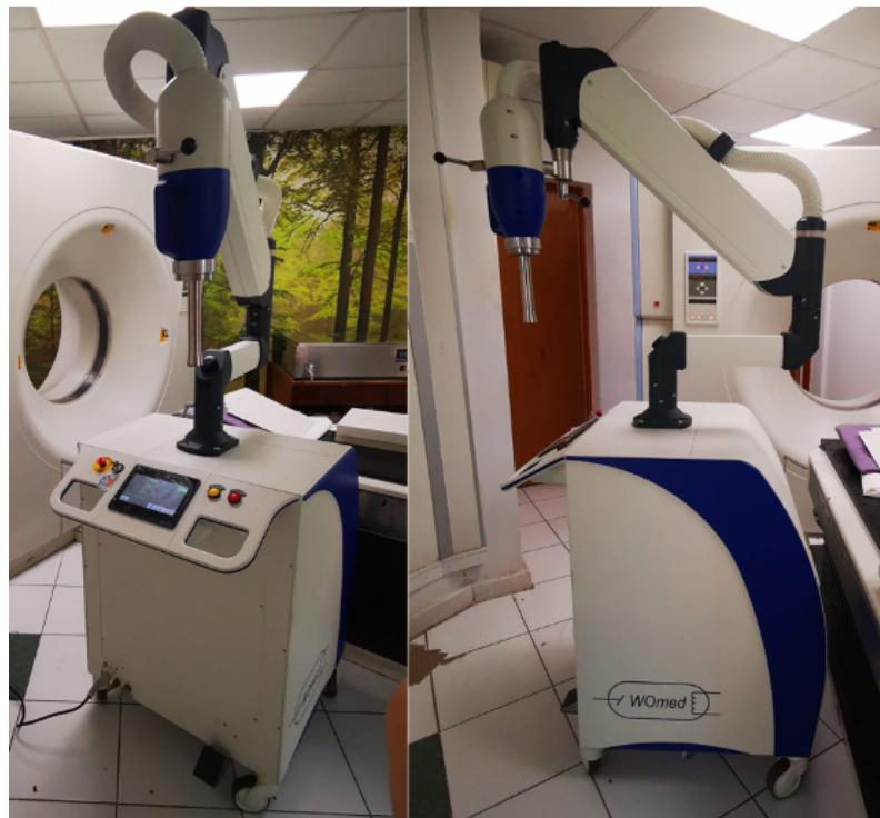
Figure 2. WOmed ioRT-50 clinical surface radiotherapy equipment used in the measurements.
