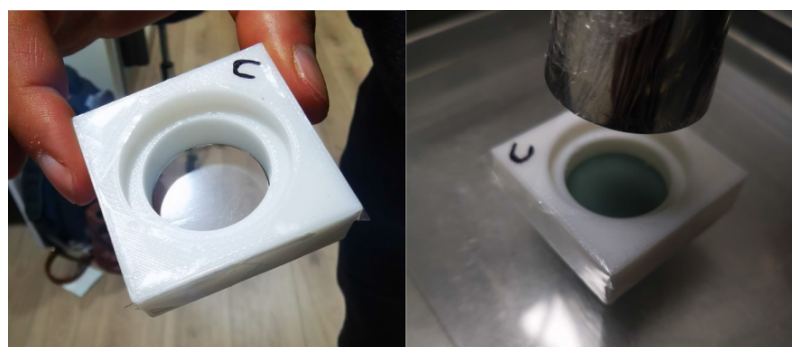
Figure 4. PMMA phantoms sealed with 2.5 \mu\text{m} and 12 \mu\text{m} Mylar films to contain a 6.15 \text{cm}^3 suspension volume deposited on delaminated EBT3 film dosimeters.
