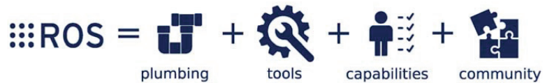
Figure 1. The ROS ecosystem is composed of multiple elements: (i) plumbing: a message-passing system for communication; (ii) tools: a set of development tools to accelerate and support application development; (iii) capabilities: drivers, algorithms, user interfaces as building blocks for applications; (iv) community: a large, diverse, and global community of students, hobbyists and multinational corporations and government agencies.
