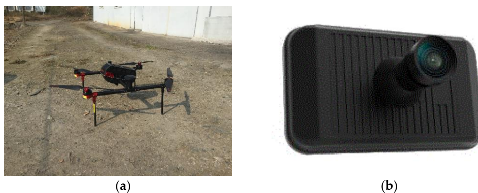
Figure 3. (a) The Feima UAV platform; (b) the SONY a-6000 digital camera.
