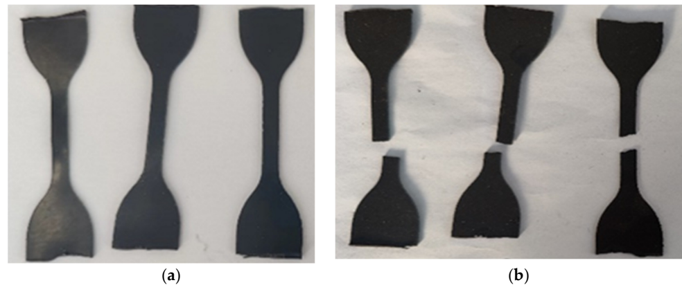
Figure 16. Tensile test specimen: (a) shape before tensile test; and (b) shape after tensile test.
