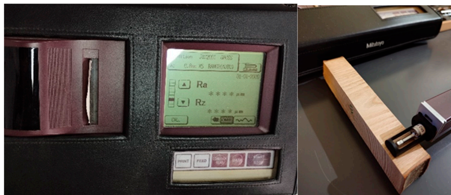
Figure 3. Profilometer device and view of surface roughness measurements on wood on the right.
