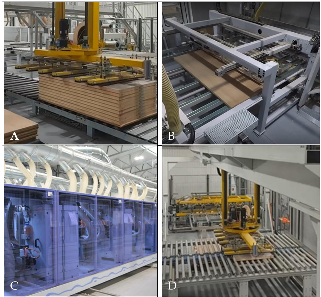
Figure 2. The units of the edge banding module: (A) feeding portal, (B) reference milling machine, (C) edge processing machine, (D) two-way stacking portal.
