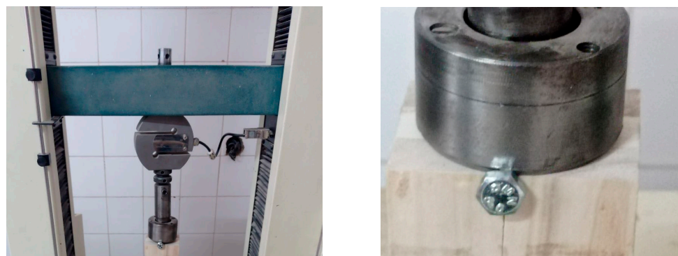
Figure 3. The loading apparatus of CLT samples for embedment strength testing.
