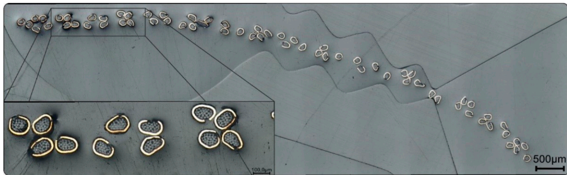
Figure 5. Cross-section image of the High Flex 3981 braided ribbon. In the zoom window, the individual yarns covered with thin silver-plated copper foil are shown for better visualization.
