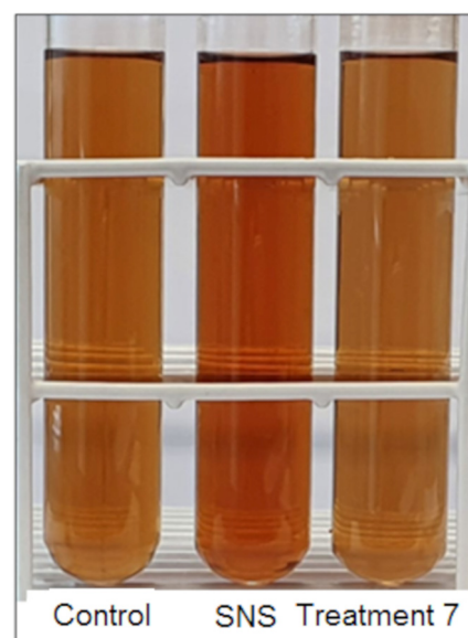
Figure 3. Residual dyeing solution: control, SNS and treatment 7—130 °C.
