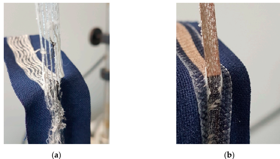
Figure 10. Visual fracture determination of the samples after the peel tests: (a) mixed fracture for Amotape 3587; and (b) adhesion fracture for High Flex 3981 prelaminated with TPU.
