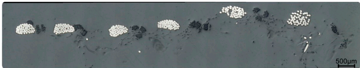
Figure 6. Cross-section image of the Amotape 3587 woven ribbon with six parallel-running bundles of silver-plated copper strands. The Amotape 46050 woven ribbon with six crossed bundles of silver-plated copper strands and additional hotmelt yarn is not displayed as the cross-sections of both Amotape versions are comparable.
