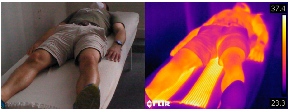
Figure 22. A 90 cm × 190 cm knitted bed sheet with integrated Y08 yarns, ultrasonically welded with conductive ribbon Elasta Vestil as a continuous contact element for the interconnection of the heating yarns.
