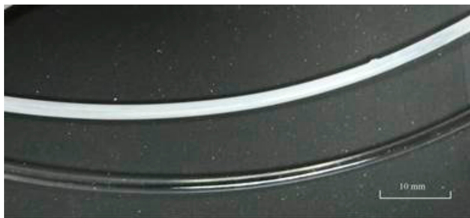
Figure 1. The appearance of PETG polyester sample before and during sorption of acetic ester.
