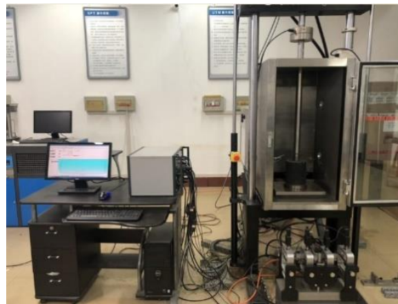
Figure 2. Uniaxial penetration test device.
