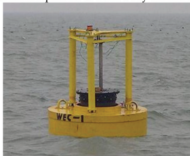
(b) Double-buoy OW ECS in ocean waves
