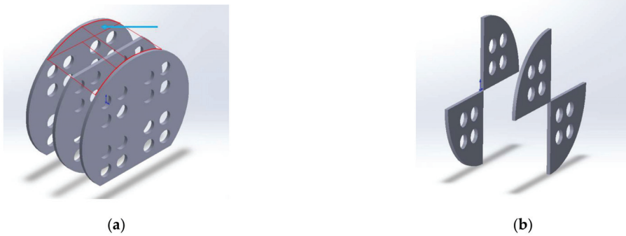
Figure 3. Single-curved baffle and flower baffle in shell and tube heat exchanger. (a) Single-curved baffle, (b) flower baffle.
