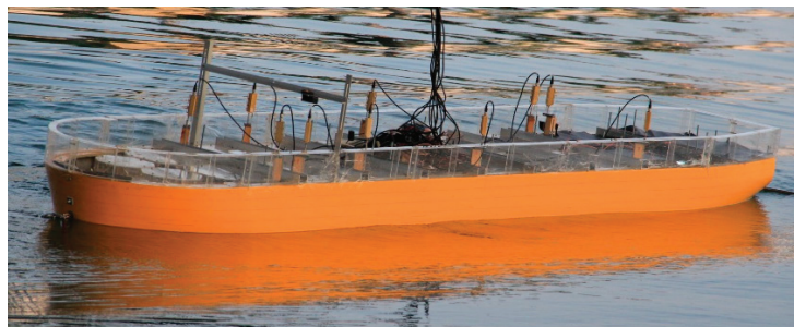
Figure 3. Aquaculture vessel model in the basin.
