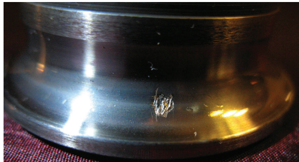
Figure 2. Material loss on the inner race of the bearing.
