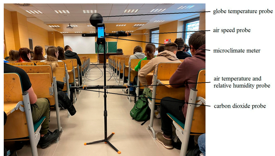
Figure 2. The microclimate meter with the probes.
