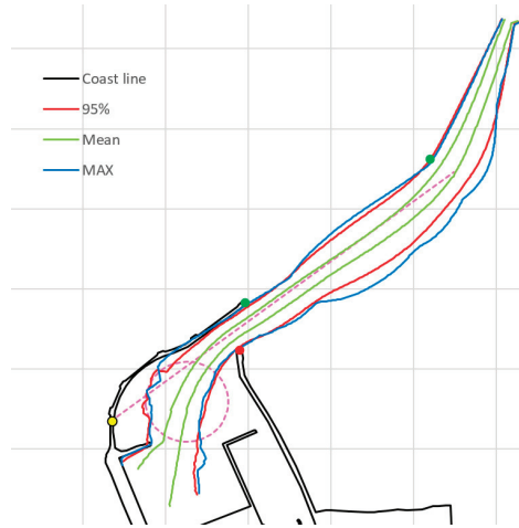
Figure 12. Manoeuvring areas of a general cargo ship of L = 133 m on approach to modernized Ustka Port by “Soft-Bank” with limited (preliminary) navigational marking.
