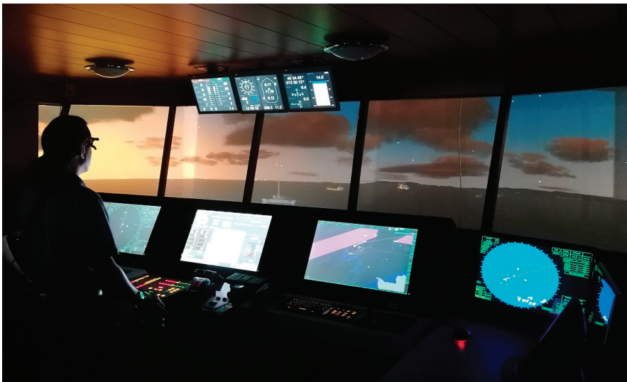
Figure 1. Full mission simulator: Experienced participant during collision avoidance in the traffic separation zone wearing pupil-diameter sensor and wrist multi-sensor.
