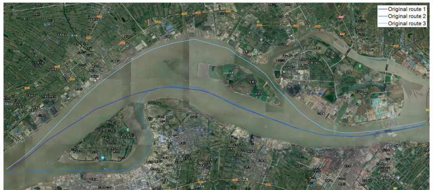
Figure 19. Original AIS trajectory map (three typical trajectories).
