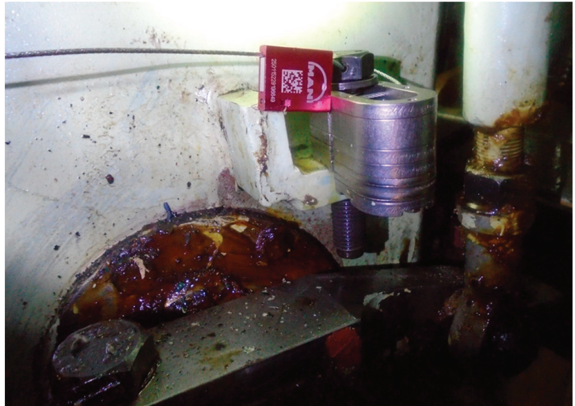
Figure 1. Engine power limiter of a mechanically driven type engine (changing a set of governor’s fuel index).
