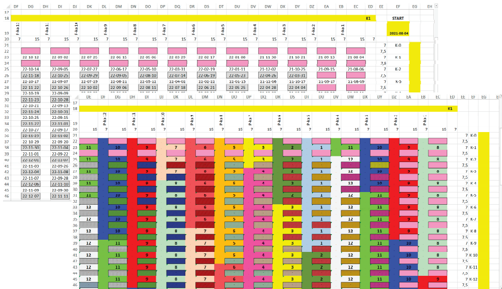
Figure 7. Planned schedule of mining works in the room and pillar mining system.
