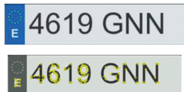
Figure 10. Image of a license plate and the image processing performed detecting feature points.
