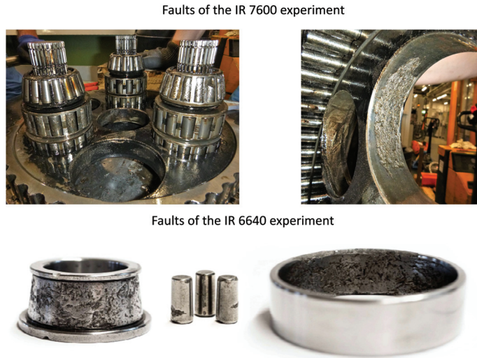
Figure 5. Overview of the faults of the accelerated wear tests following [3,39].
