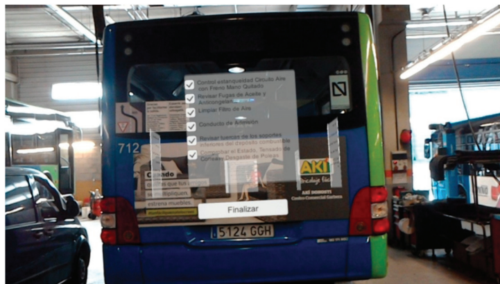
Figure 12. Example of an AR panel showing it through the HoloLens device.
