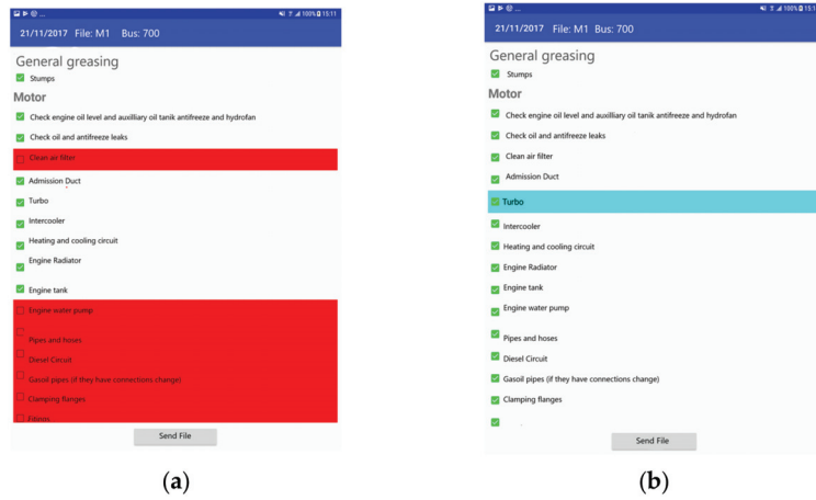
Figure 4. Maintenance sheet M1 with unedited field (a) and maintenance sheet M1 with incident notification (b). Red background marks not yet started tasks and blue background marks reported tasks.
